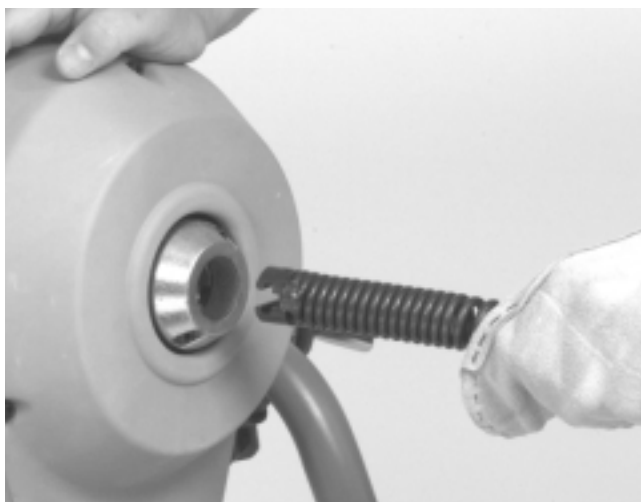
Figure 4 – Inserting Cable Into Front Of Machine
