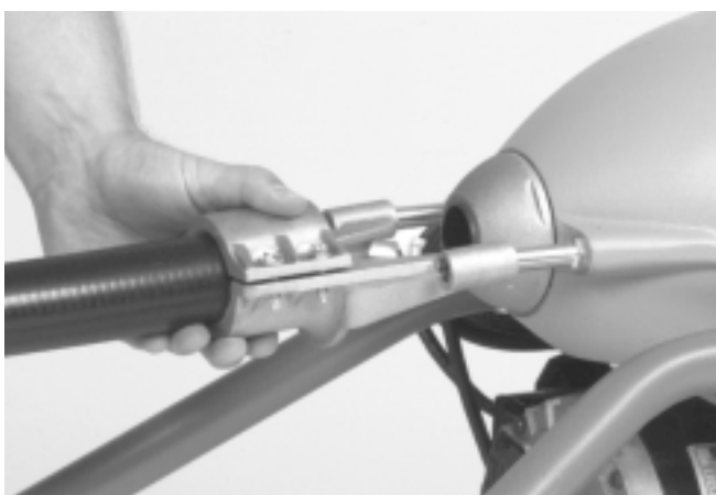
Figure 3 – Rear Guide Hose Attachment
