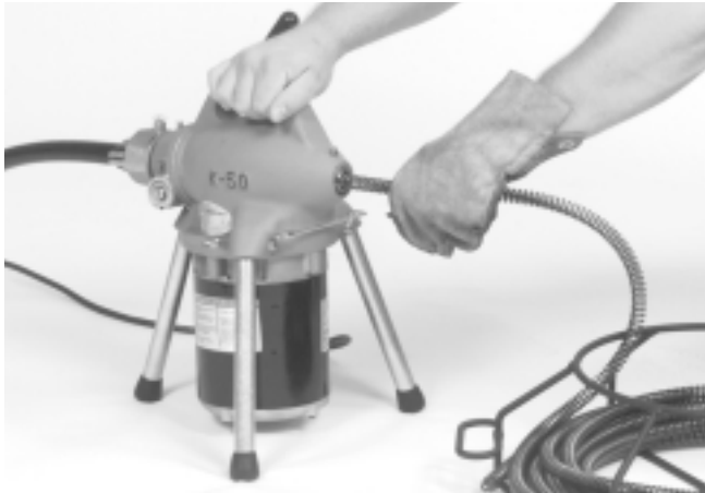
Figure 3 – Inserting Cable Into Front Of Machine
