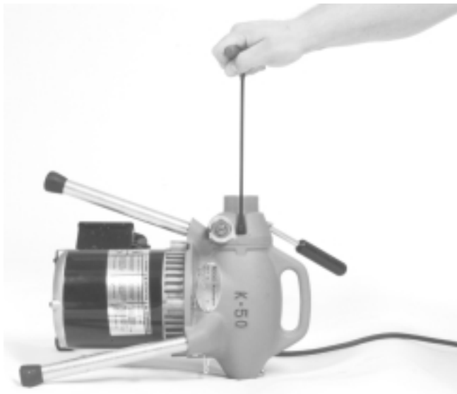
Figure 10 – Remove Socket Head Cap Screws
