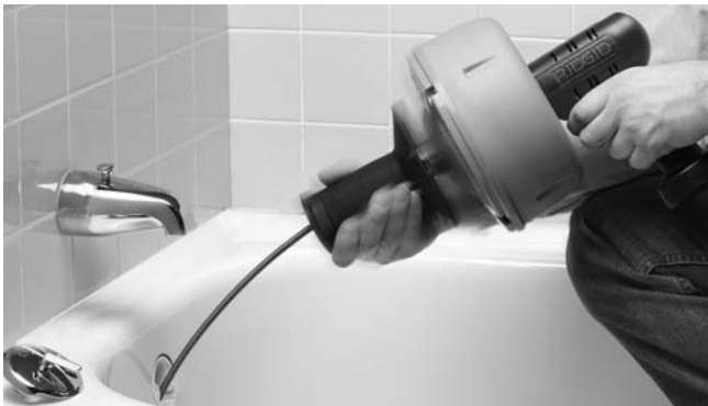
Figure 7 – Pull Handgrip FORWARD To Disengage Clutch and Draw Additional Cable From Canister
