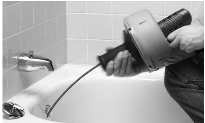
Figure 5 – Pull Hand Grip Rearward To Engage Clutch
