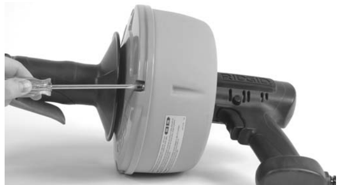
Figure 9 – Loosen Four (4) Screws From Back Half of Canister About Three (3) Full Turns
