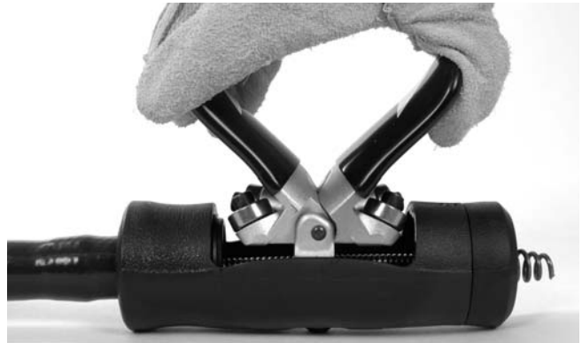
Figure 5 – Feeding cable through AUTOFEED
