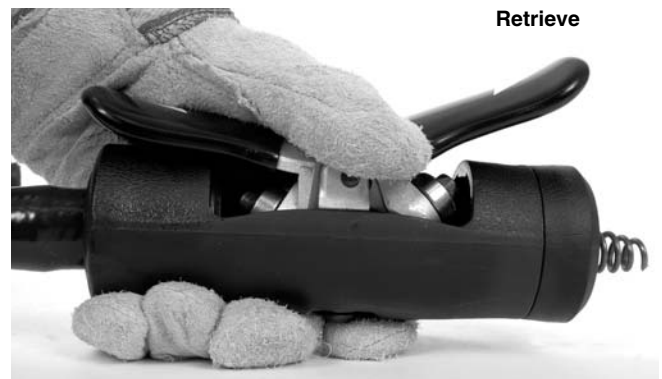
Figure 15 – AUTOFEED in Advance and Retrieve Position
